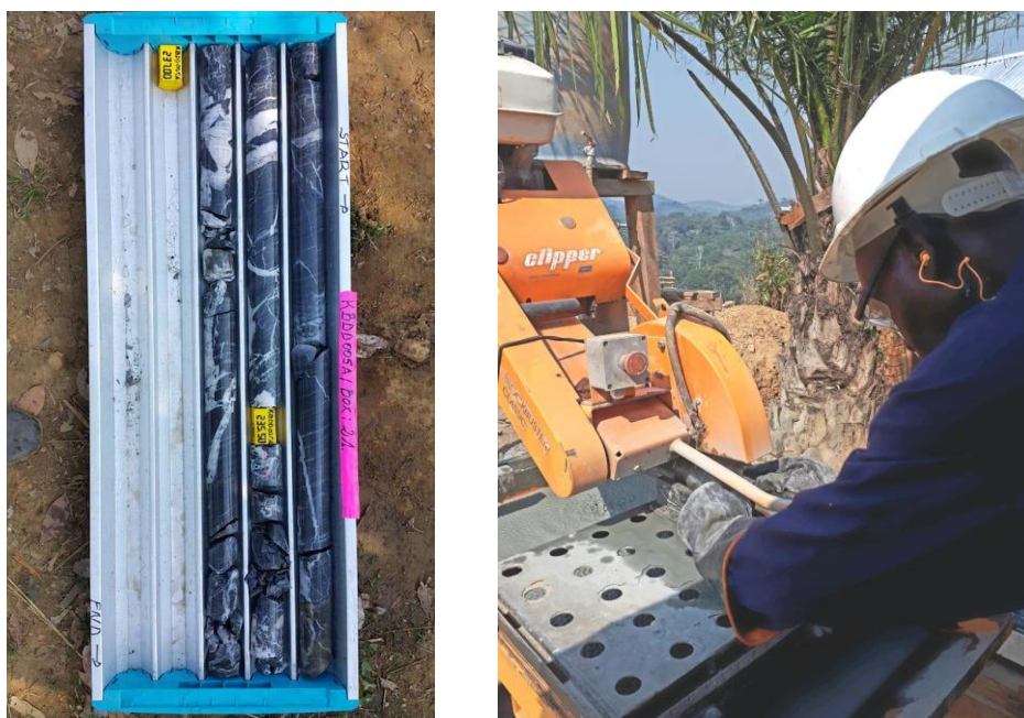
Figure 15 and 16: K235m Carbonaceous Schist with quartz veins and minor sulphide AND core cutting KBDD005A collared nearby at a steeper angle to reach the designed target and cementation allowed the hole to be completed to plan. A series of zones with sulphide and quartz vein were intersected between 160-260m.
