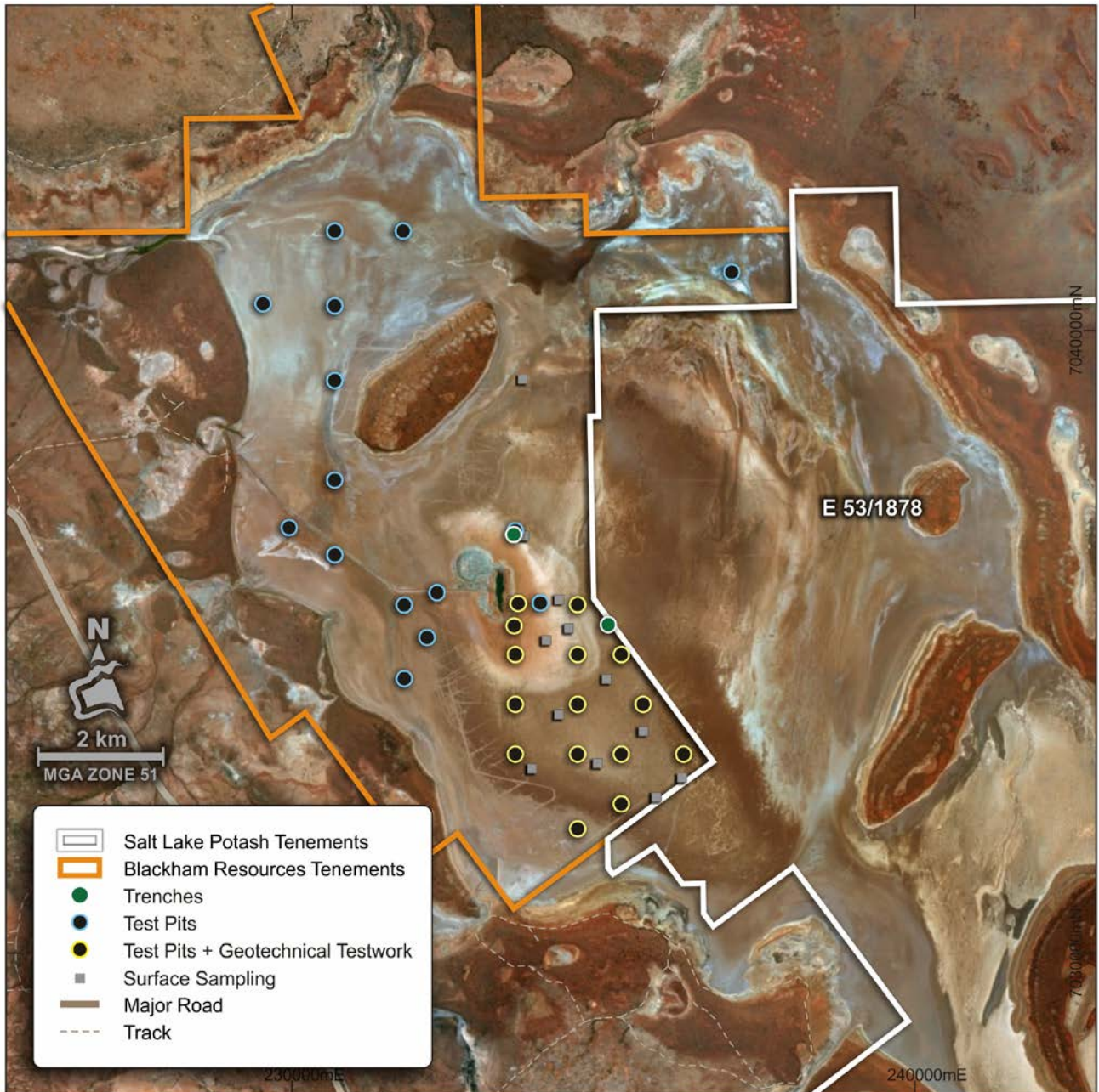
Figure 12: Surface Aquifer Exploration Program
