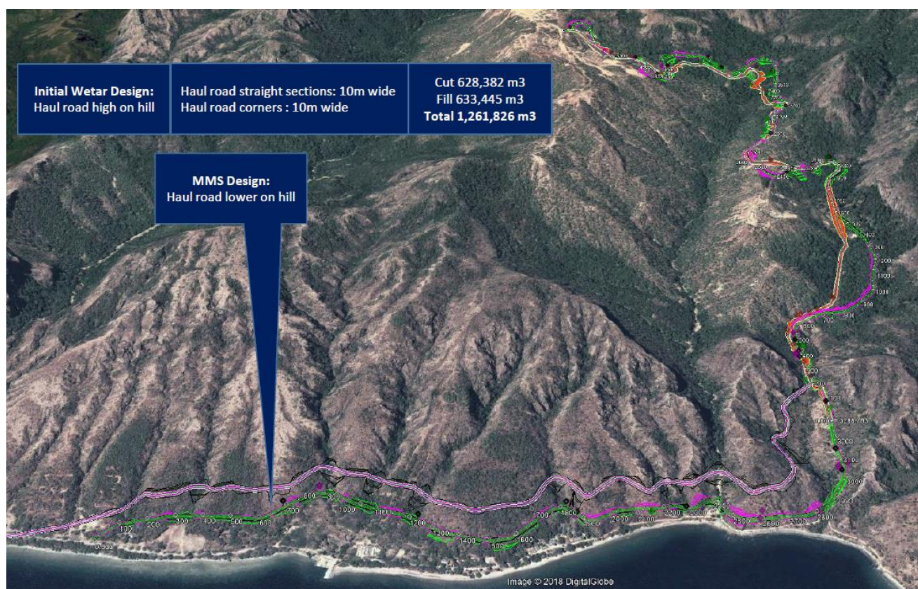
Figure 4– Original Lerokis haul road (pink) and the optimised route (green).
