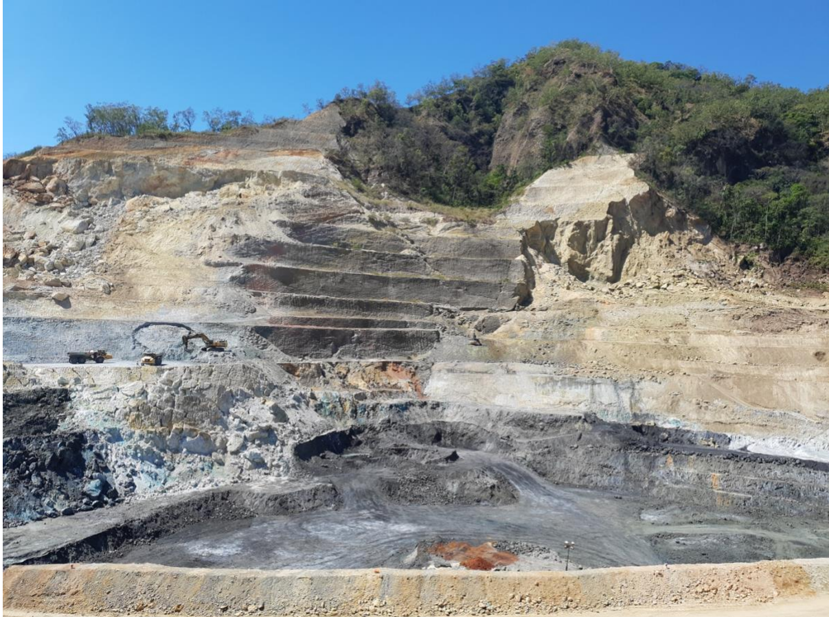
Figure 1 – Kali Kuning open pit with north wall slip remediation in action
