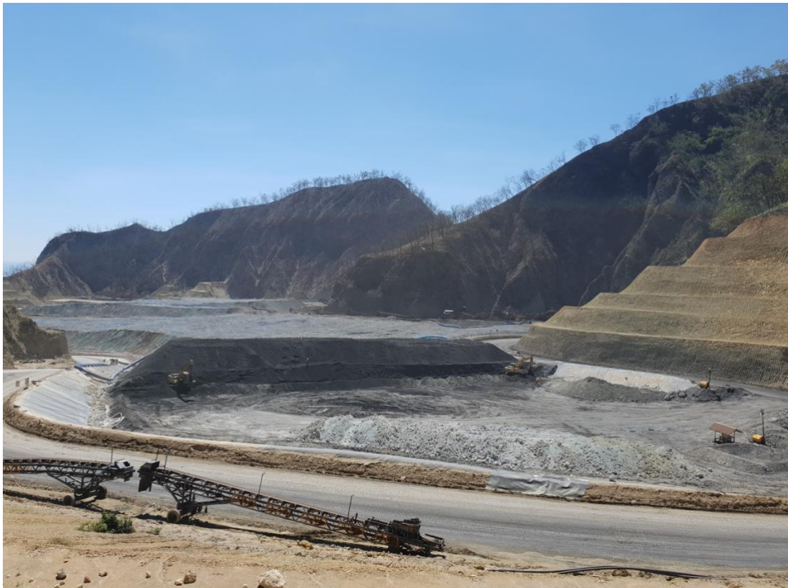
Figure 2 – Leach pad KK06 being stacked with ROM Fresh Ore.
