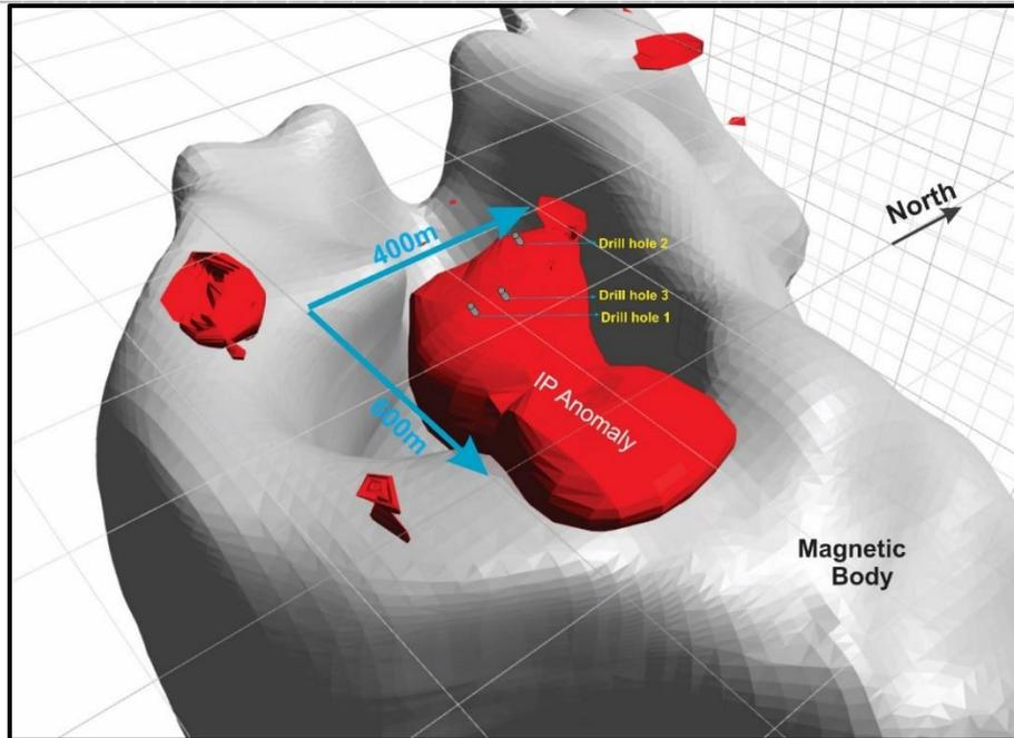
Figure 1: 3D Chargeable IP Anomalies with Drill Targets
