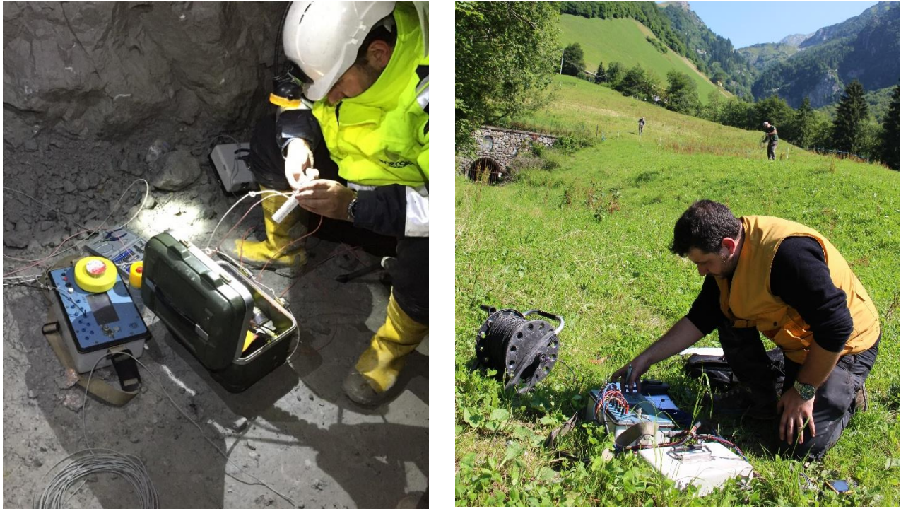
Figure 7: Resistivity survey underground and surface activity
