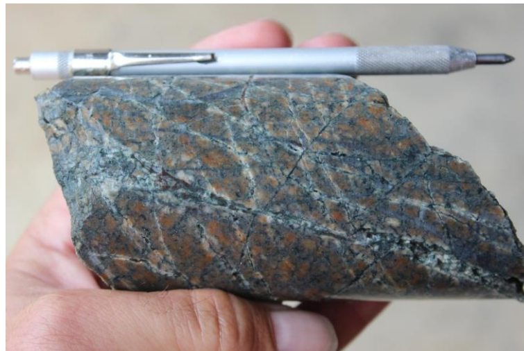
Photo 5. Quartz-magnetite \pm hematite 'M' veins in a hematite altered quartz diorite porphyry at 272m in SMD025.
