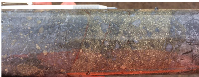
Photo 7. Breccia with pyrite clasts and later bornite veining at 580.8m in SMD028.
