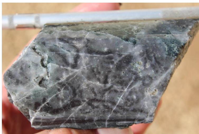
Photo 3. Quartz-magnetite ± pyrite ± chalcopyrite veining at 441m in SMD024.
