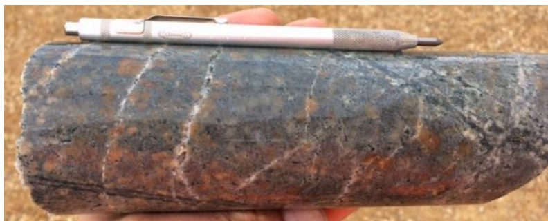
Photo 6. Hematite altered quartz-diorite porphyry with fine disseminated magnetite at 530m in SMD028.
