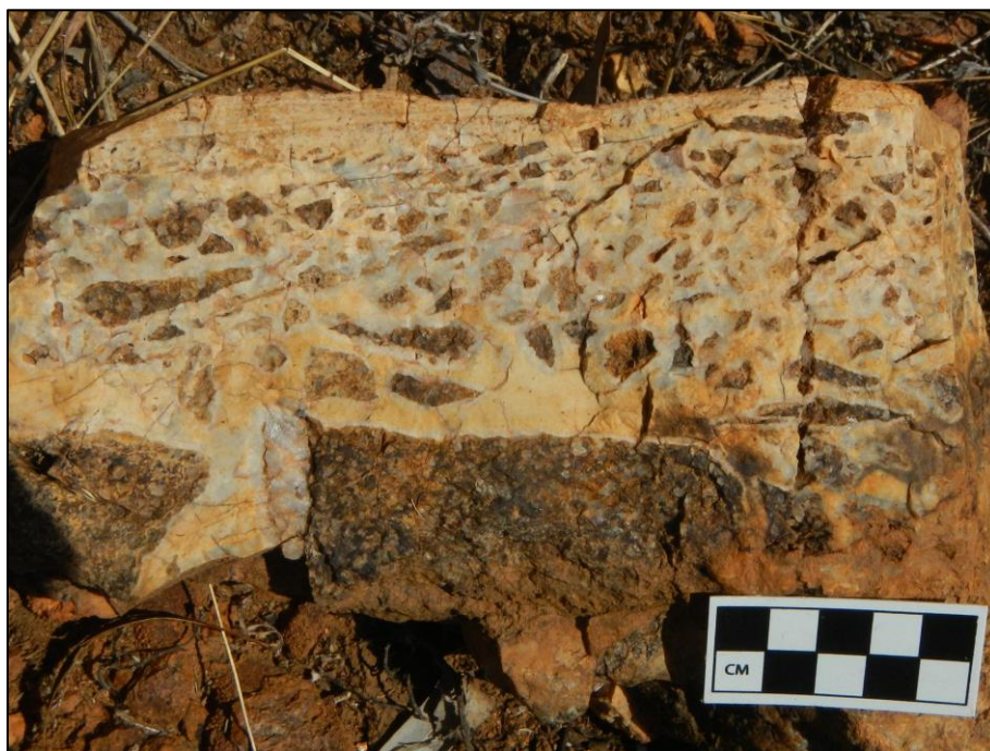
Photo 10. Quartz-carbonate breccia vein with crustiform quartz then carbonate surrounding angular clasts of rhyolite / volcaniclastic sandstone - 0.55 g/t gold and 62 ppm antimony.
