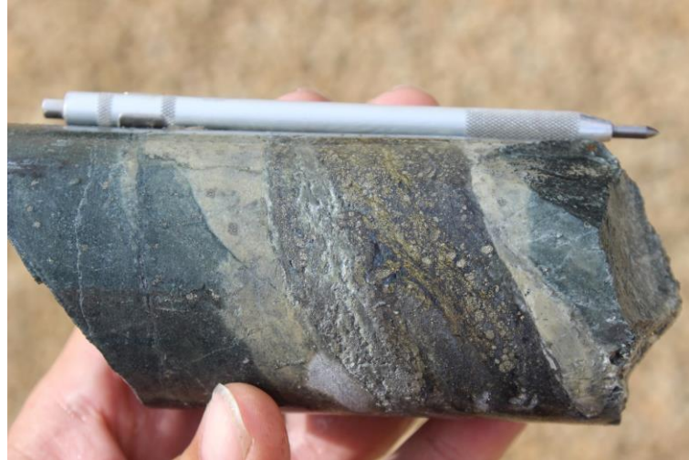
Photo 4. Pyrite \pm chalcopyrite \pm chalcocite vein at 151.9m in SMD025.
