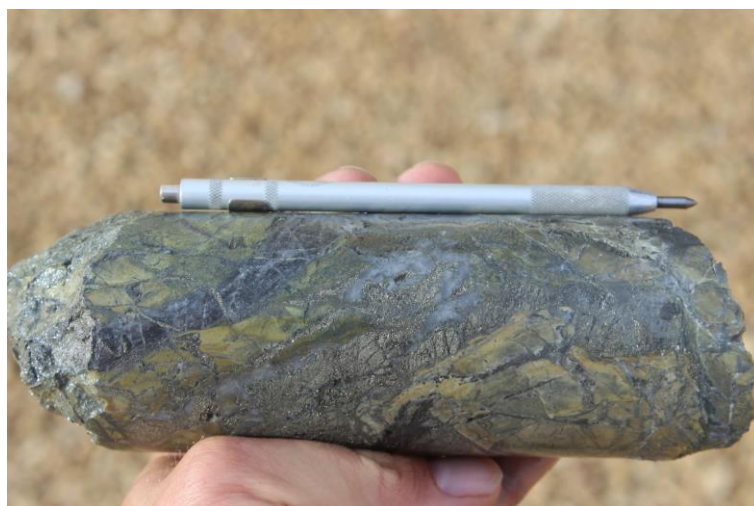
Photo 2. Quartz-magnetite ± pyrite ± chalcopyrite veining being cut by later pyrite veins at 399.5m in SMD024.
