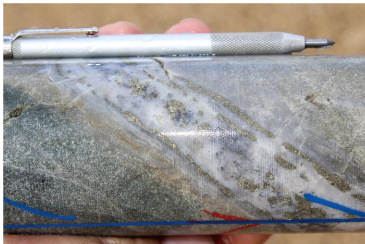
Photo 1. Quartz-pyrite-molybdenite 'D' vein at 332m in SMD024.
