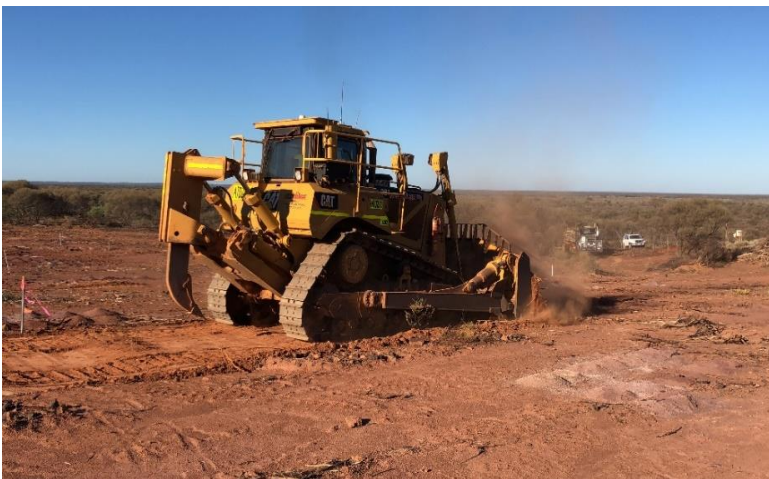
Image 2 – Dozer pushing up Bulk Sample at Barrambie
