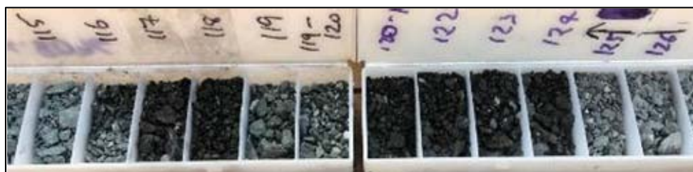
Photo: Pulses of massive and semi-massive sulphide in silica-rich units in MURC001 surrounded by highly altered volcanics; also correlated well with the DHEM plate position.
