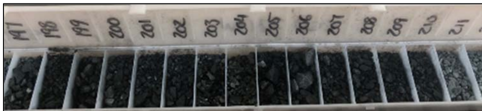
Photo: Zone of massive and semi-massive sulphide in a silica-rich unit (probable exhalite) in MURC002; zone correlates well with the DHEM modelled plate position.
