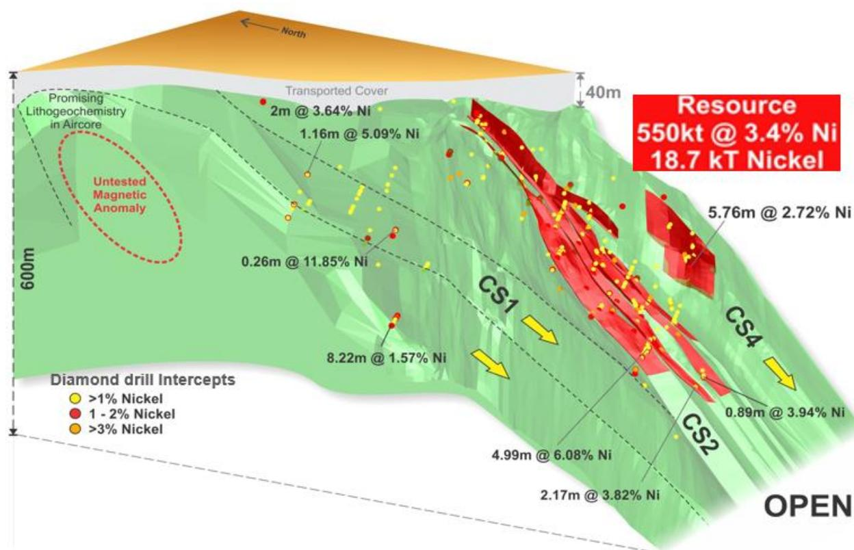
Figure 1: Growing Resource potential of the Cassini mineralised system. 3D representation of the Cassini basal contact shown in green. The CS2/ CS4 channel trends remain open and have returned high grade intersections in the last line of drilling demonstrating the strong likelihood for Resource extensions. In parallel, highly promising open-ended drilling results in adjacent channel trends points to excellent opportunities to pursue separate Resource additions<sup>2</sup>.
