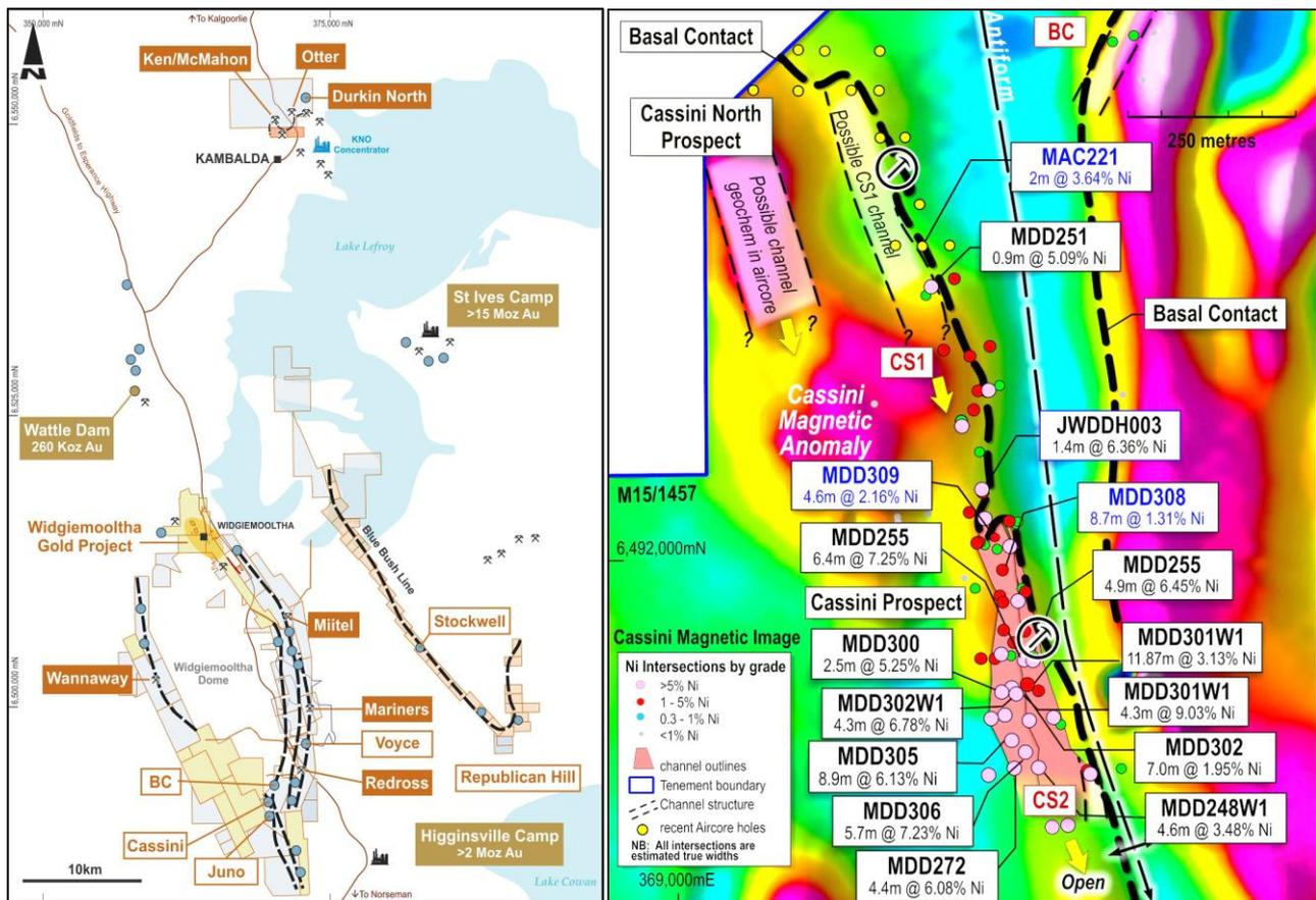
FIGURE 2: A) Mincor landholdings centred around Kambalda; B) Cassini high-resolution magnetic image showing the CS1 and CS2 channels, magnetic anomalies and numerous quality drill intersections (estimated true width)<sup>2</sup>
