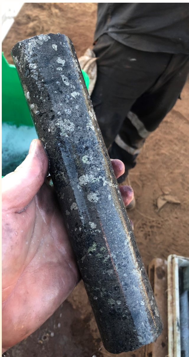
Figure 3. Brecciated massive sulphide interval from Zone 1 DMDD0015 312.28 – 312.52m downhole
