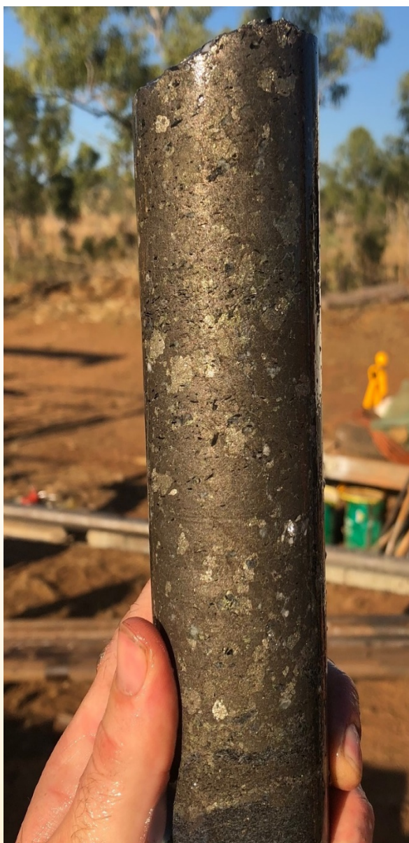
Figure 4. Massive sulphide from Zone 3 DMDD0015 342.2 – 342.46m downhole
