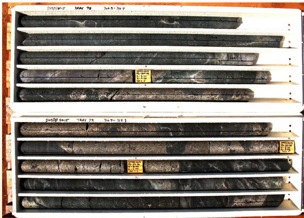
Figure 2. Brecciated massive sulphide interval from DMDD0015, core is NQ, from 306.5-315.3m downhole.
