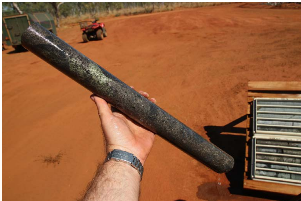
Figure 1. Brecciated massive sulphide from DMDD0015 with visible Pentlandite, Chalcopyrite & Pyrrhotite, photograph is of NQ whole core, 310.25-310.72m downhole.
