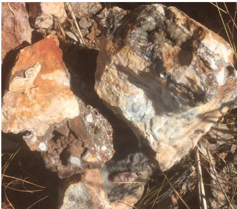
Figure 3: Breccia vein 2m wide with colloform-coxcomb textures – rock chip results to 2.11 g/t gold (Au-As-Sb association)
