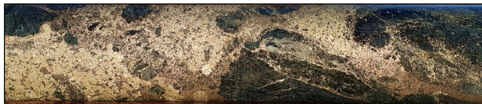
18EMDD002: 118m Pyrrhotite, chalcopyrite, +/- pyrite
