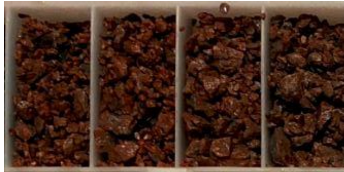
Photo 1 – NMWBRC18-010 – 204m to 208m 4m @ 2.43g/t Au. Brick-red coloured hematitic alteration at contact of high level porphyry intrusive and volcanic host rock.
