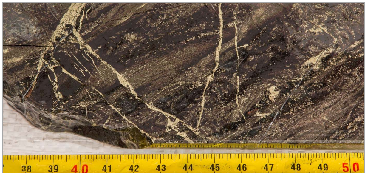
Figure 1. Visible copper sulphides and magnetite in half-core, hole ZX-18025, 94.0m down-hole depth. Copper sulphides comprise mainly chalcopyrite (yellow colour) with minor bornite . Early disseminated chalcopyrite has been overprinted by later, fracture-controlled chalcopyrite veins. Scale bar is in cm.
