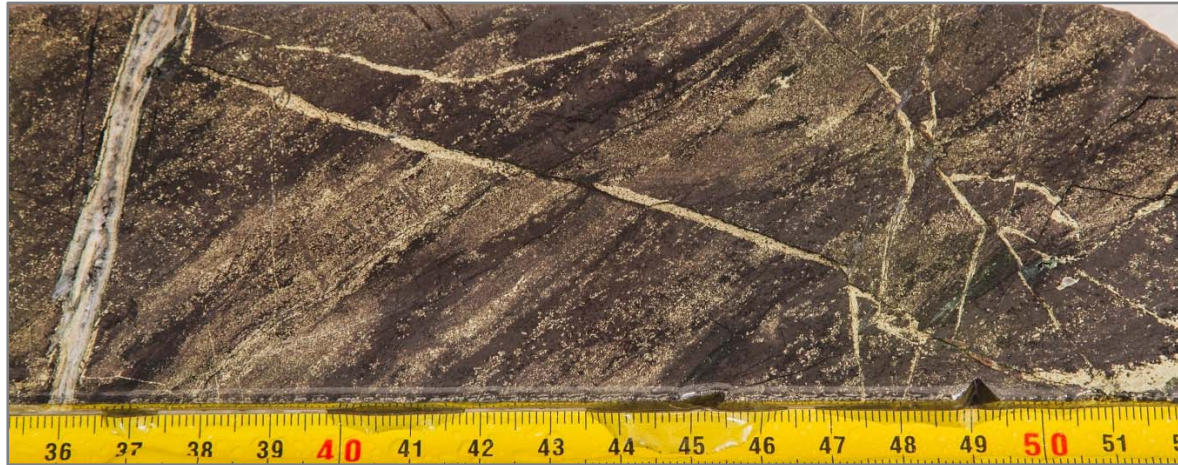
Figure 2 Visible chalcopyrite and magnetite in half-core, hole ZX-18025, 93.8mm to 94.0m down-hole depth. Scale bar is in cm. Note overprinting fracture-controlled chalcopyrite mineralisation.
