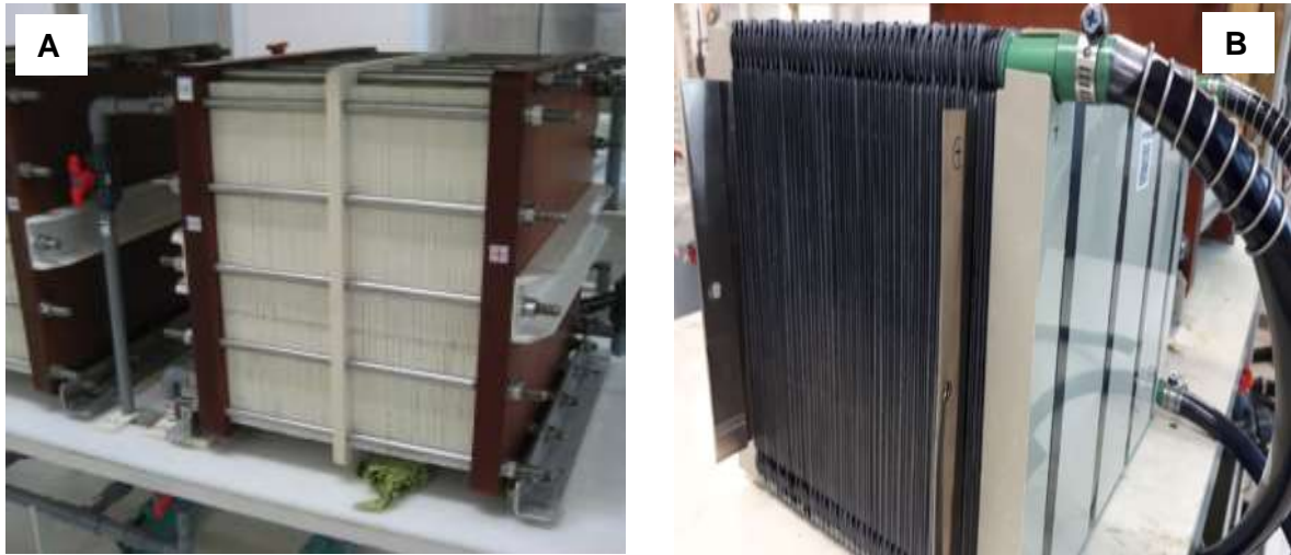
Figure 2 A: Existing battery stack technology (12.5kW stack), B: new laser welded stack (12.5kW stack)
