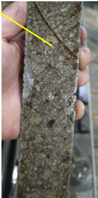
Image One | Historic Kingsley Drill Core with massive sulfides
