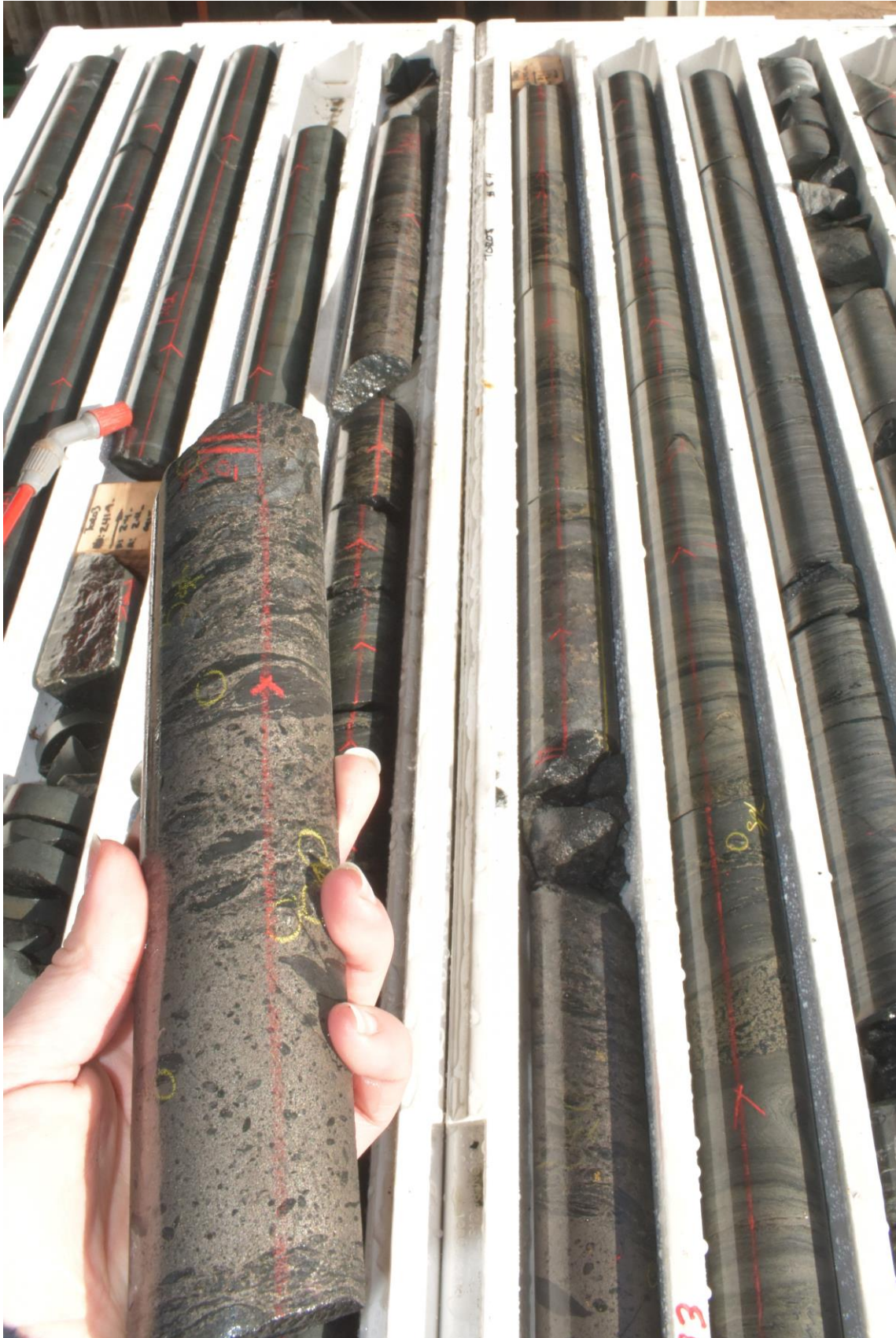
Figure One | Massive Sulfide in Drill Core from Drilling at the Thor Prospect
