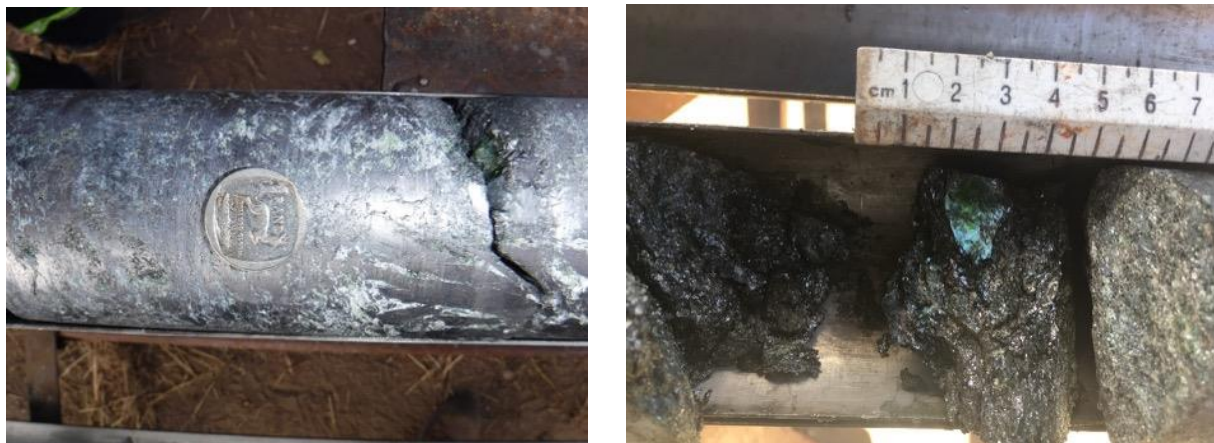
Figure 7. Large flakes intersected in MOD042 & Large roscoelite flake intersected at MOD045
