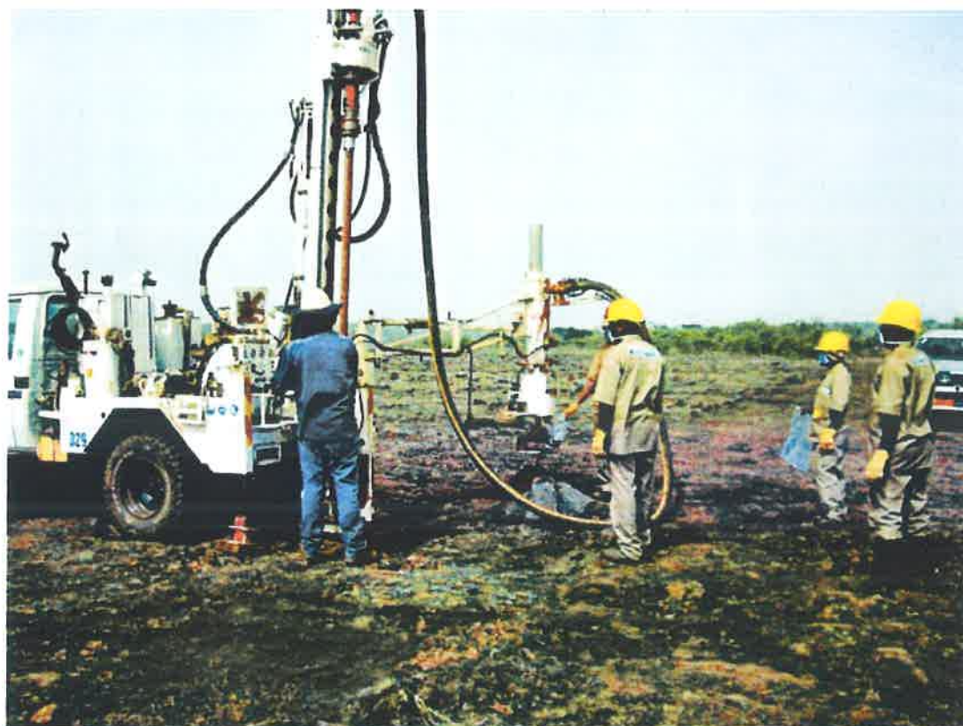
Figure 3-16: Air Core drilling and sampling on Simone Plateau by Wallis Drilling
