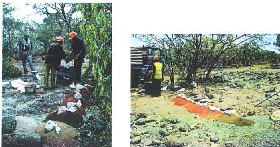
Figure 4-1: Sample splitting and collection in double bags by Labogenie at Minim Martap
