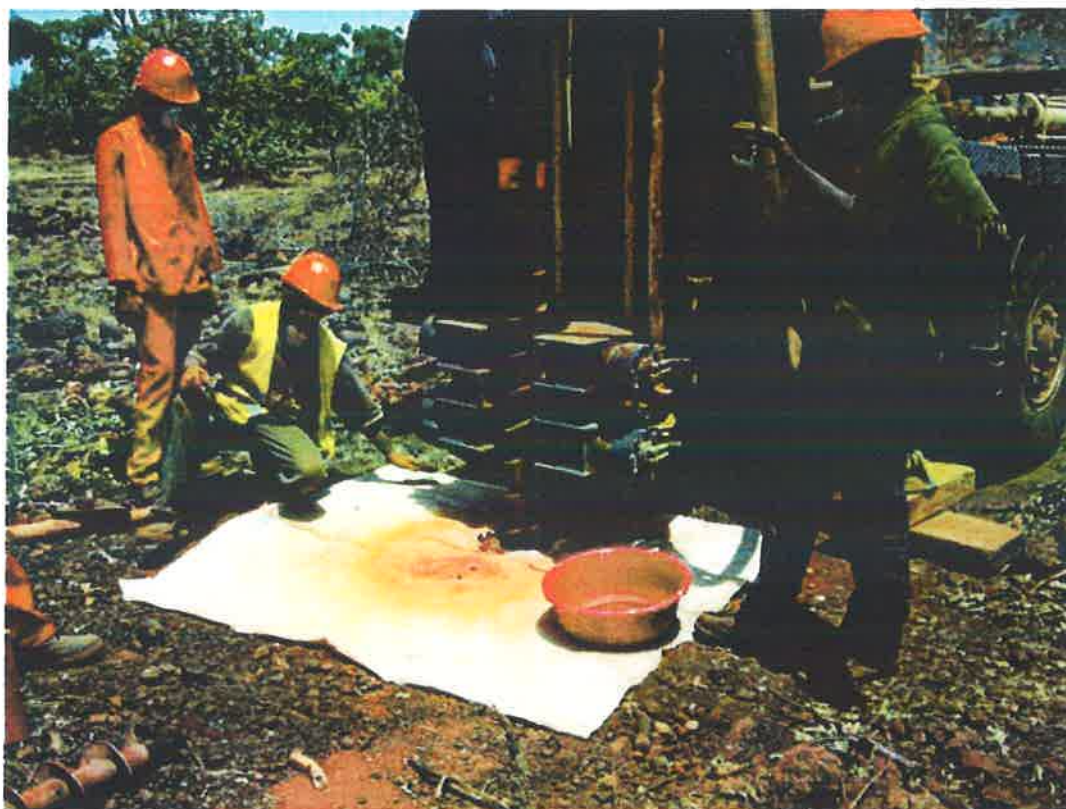
Figure 3-15: Auger drilling on Gilberte Plateau by Labogenie
