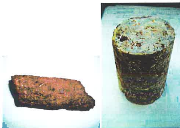
Figure 5-38: Core samples from Simone and Danielle considered the more dense bauxite (for measurements see Table 2-14)
