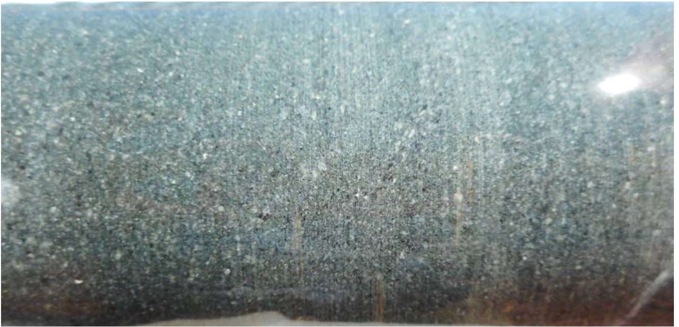
Plate 4 Detrital pyrite in sericite-chlorite alter pebble to cobble conglomerate at 46.90m (core diameter 61.10mm).
