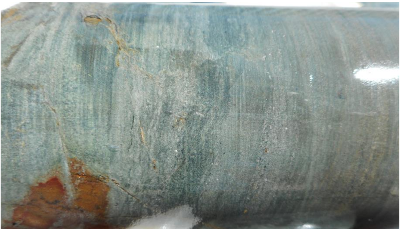
Plate 2 Chlorite altered, laminated siltstone at 27.20m (core diameter 61.10mm).
