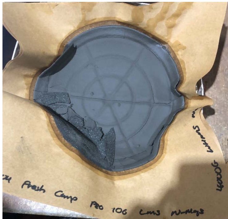
2000 G WHIMS magnetic concentrate produced from the Fresh LIMS non-mags
