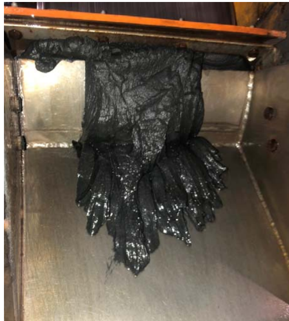
Fresh LIMS pass 2 magnetic concentrate.
