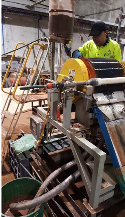
Rare Earth Drum set up showing feed, non magnetic tails and magnetic concentrate produced. Currently fed with Oxide LIMS non-mags
