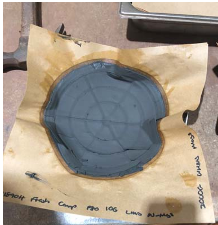
2000 G WHIMS magnetic concentrate produced from the Fresh LIMS non-mags
