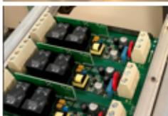
Radio switch (dual 20 amp channels)
