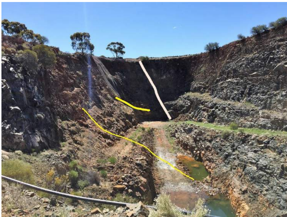
Figure 28 Mulwarrie Central pit looking North yellow is the central lode pink massive porphyry
