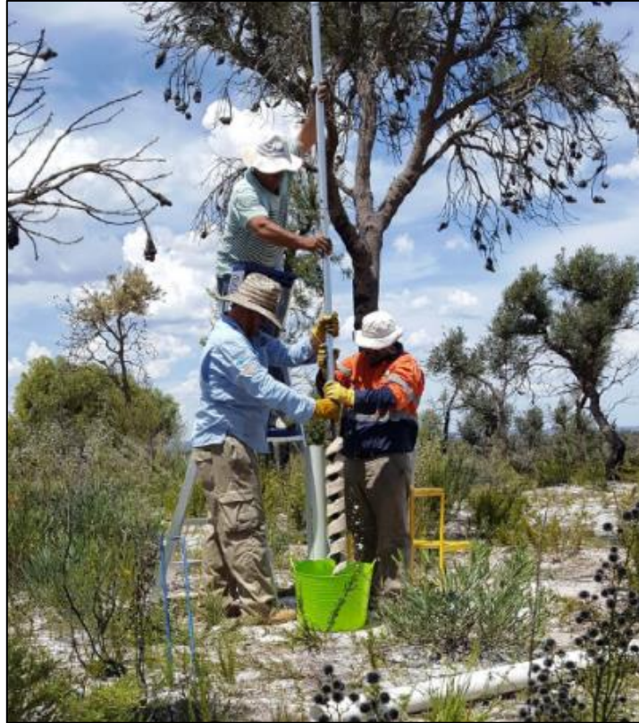
Figure 4: Sand sampling using a hand auger at Muchea
