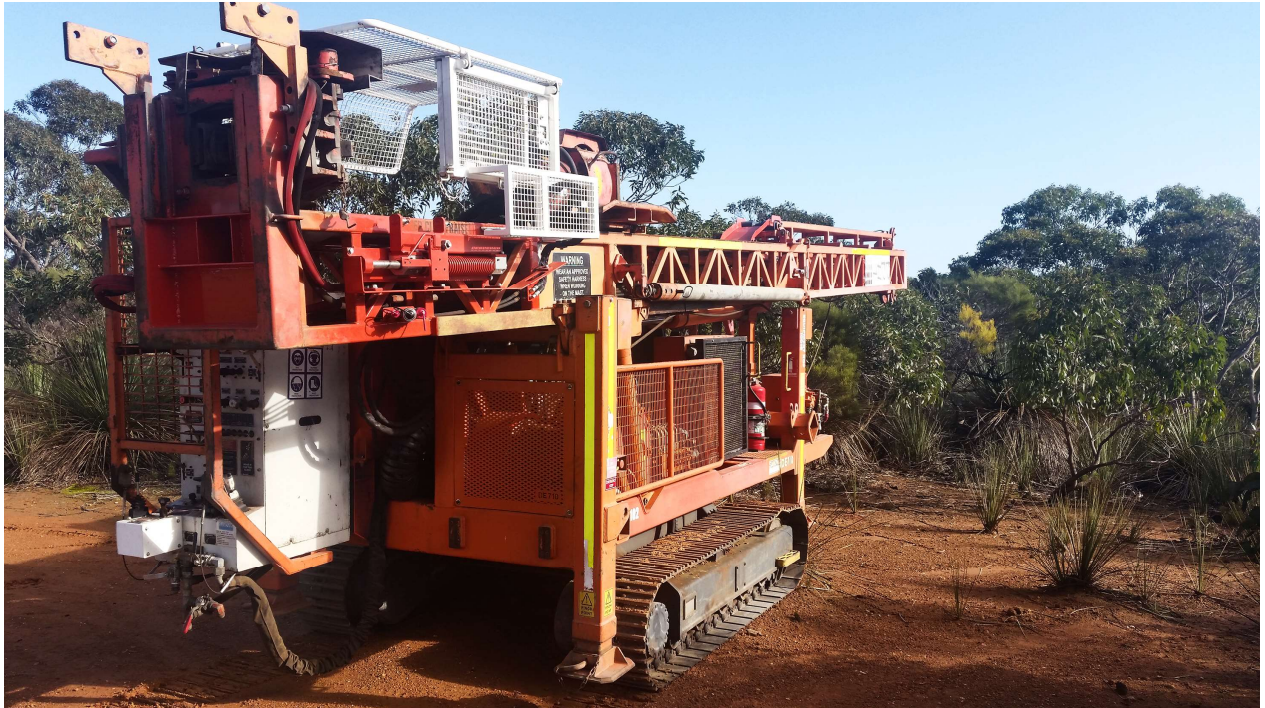
Figure 3 – DDH1 Drilling’s Sandvik DE710 diamond rig arriving on site at the Bonaventura Project.
