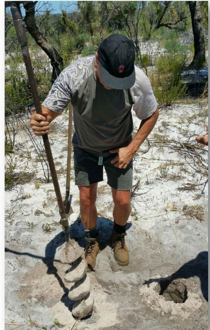
Drilling using 4WD-mounted AC rig and hand held auger
