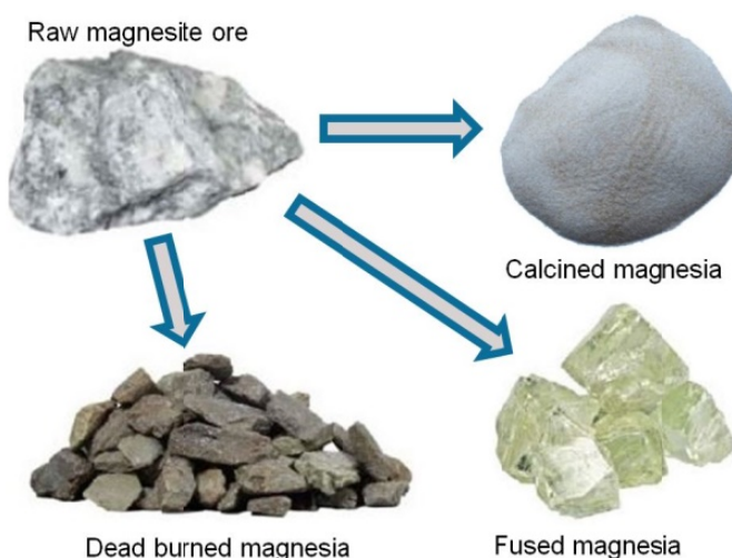
Figure 3 Raw magnesium carbonate rock processing
