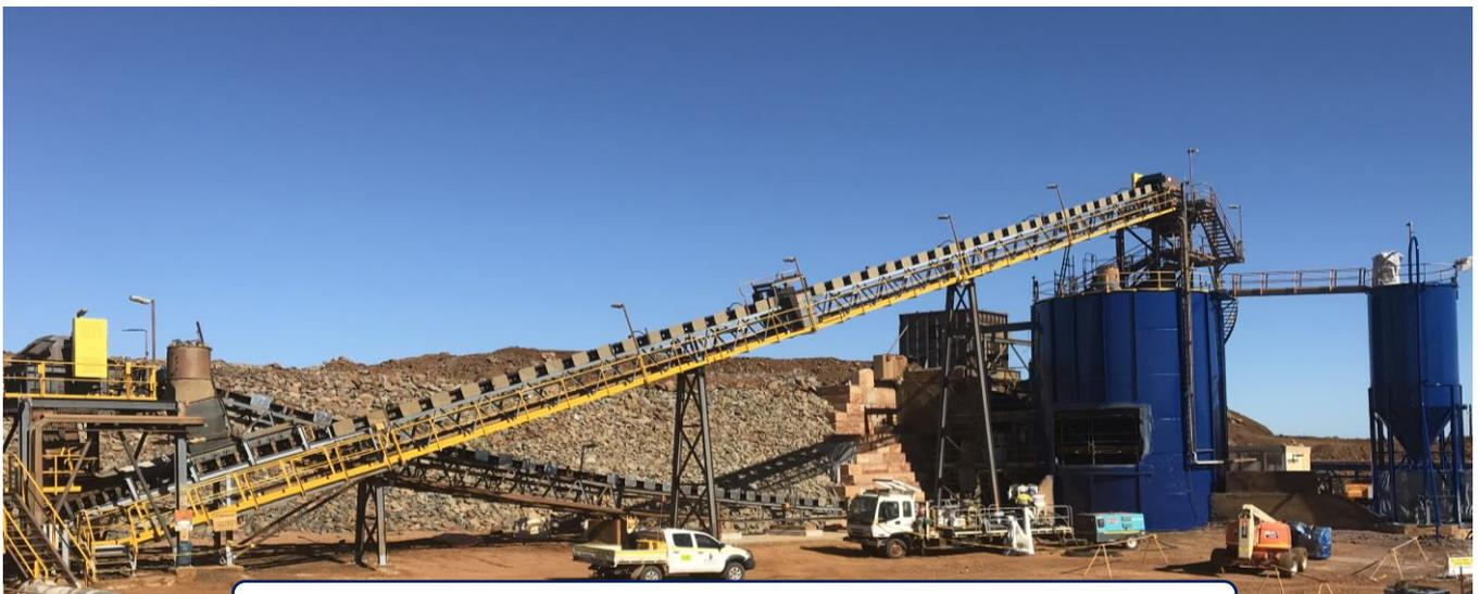
**Figure 2 – Refurbished crushing circuit and fine ore bin at Radio Hill**
