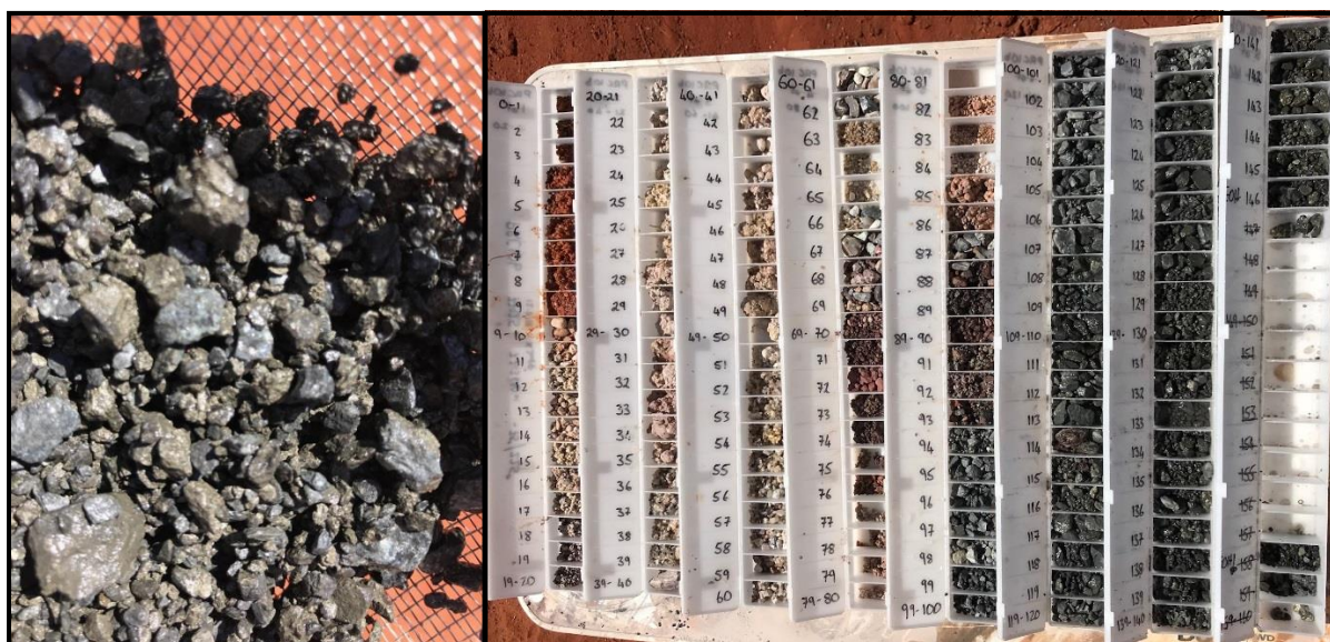
Figure 3. Sieved RC chips from 130m (left) & PRC10B 1m to 146m EOH (right)
