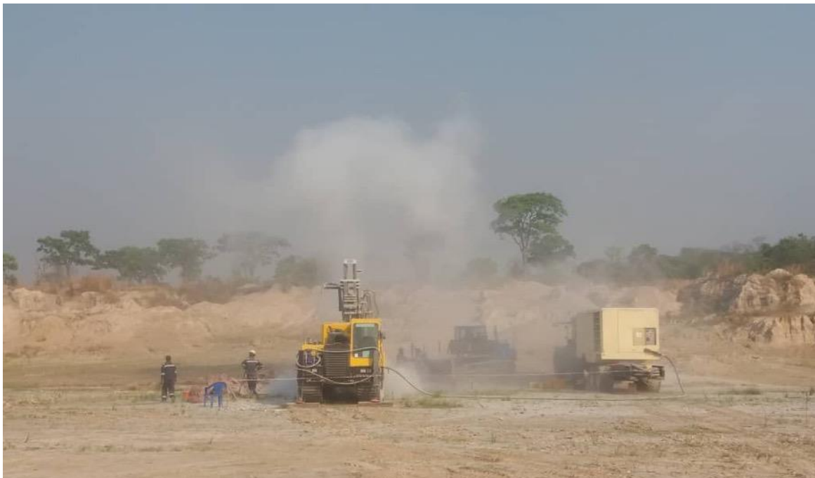
Figure 1: RC Drilling at the Kanuka Lithium Production Project in the DRC
