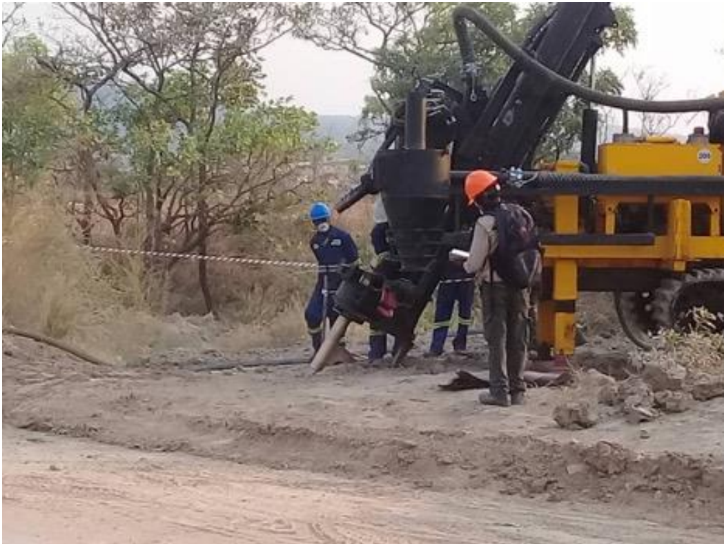
Figure 7: RC Drilling at the Kanuka Lithium Production Project in the DRC
