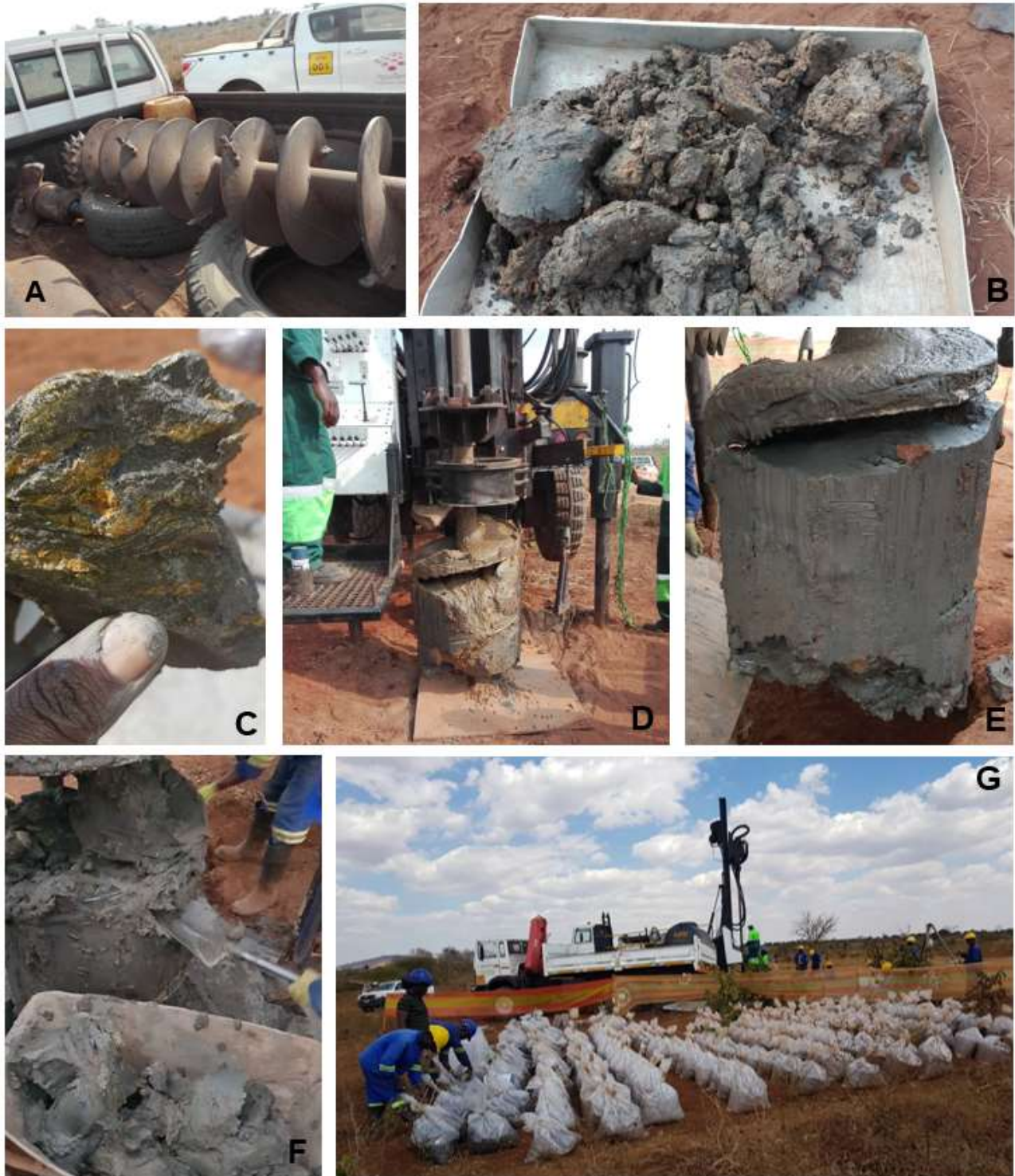
Figure 2. A – example of spiral auger bit used for bulk sampling. B- sample tray containing mineralised saprolite after removal from spiral auger bit. C – example of high grade saprolite-hosted graphite mineralisation with original foliation still evident. D – bulk sample extracted by spiral auger drilling. E – close-up of high grade saprolite-hosted mineralisation within spiral auger bit. F – removal of mineralised saprolite from spiral auger bit. G – bags containing completed bulk spiral auger samples from drill-hole MGSA0001.
