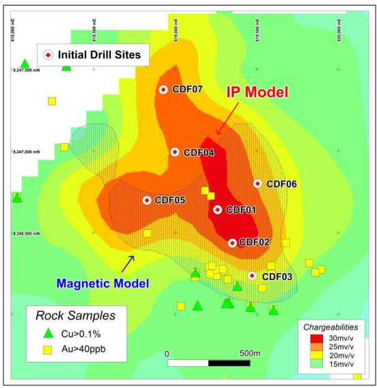
Figure 1: Cerro de Fierro IOCG target showing location of the initial drill holes.
