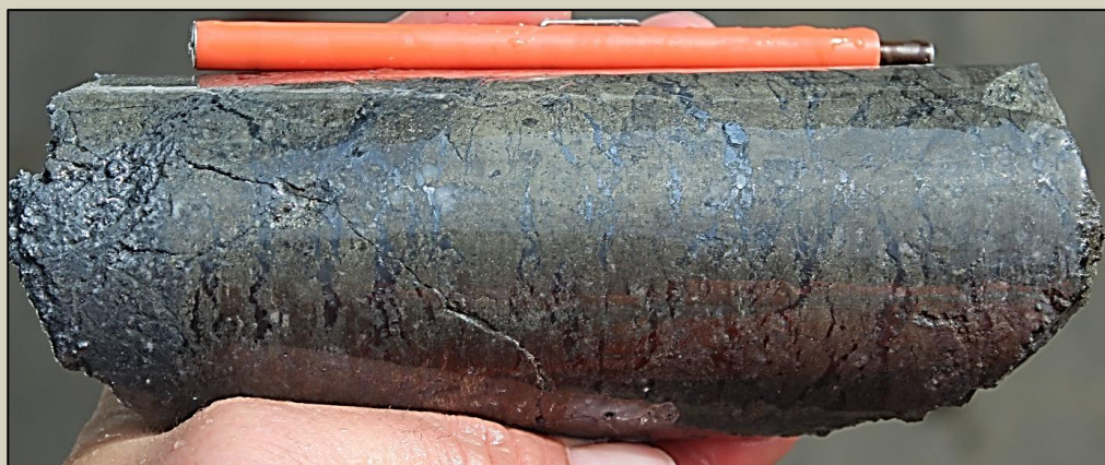
Photo 4. Massive pyrite vein with later chalcocite veining at 542.3m.
