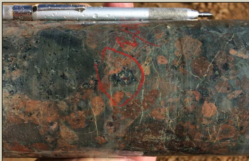
Photo 1. Hydrothermal breccia with bornite in clast at 80m.
