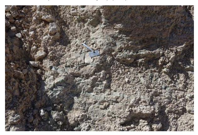
Figure 4: Hard silcrete exposed within the Cammi's Creek Pit.
