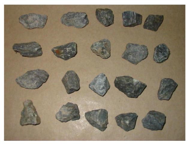
Figure 2 – A Typical Set of Particles for Breakage (Particle Selection Method)
