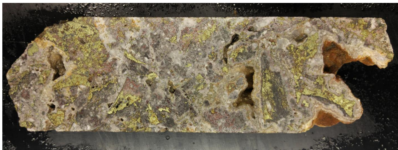
Figure 2: Drill core from FR18-004 showing chalcopyrite within brecciated skarn at 211.8m.
