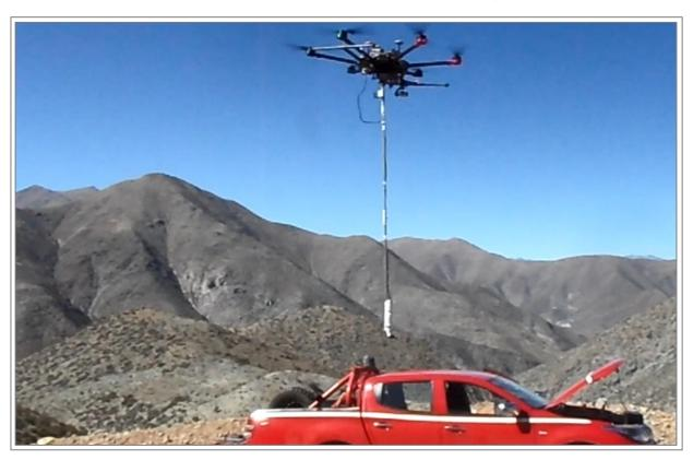
Figure 3 Drone and Aeromagnetic Sensor - Joshua Survey (in progress)
