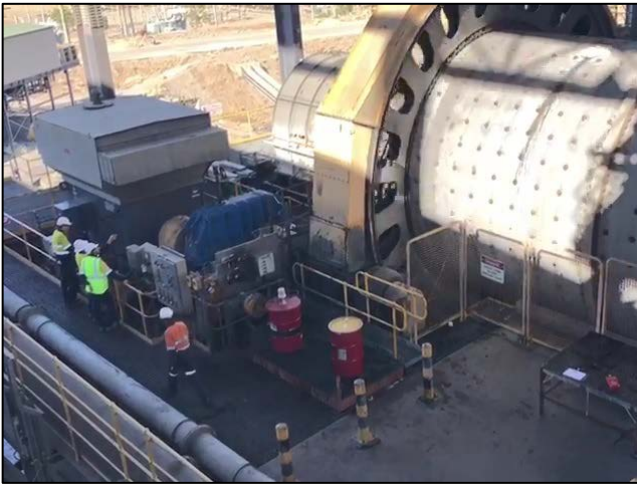
Figures 8 & 9: Ball mill (left) & fine grind mills (right) refurbished and operating within the Processing Plant
