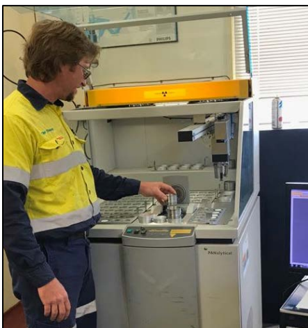
Figures 12 & 13: Laboratory Superintendent Clint Stacey operating the XRF analyser (left) & fusion unit (right) at the onsite laboratory of the Century Zinc Mine
