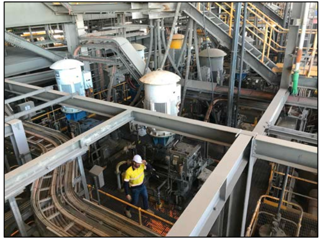
Figures 8 & 9: Ball mill (left) & fine grind mills (right) refurbished and operating within the Processing Plant
