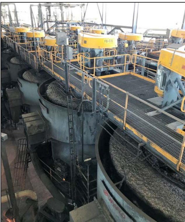
Figures 6 & 7: Flotation within the scavenger circuit (left) & production of final cleaner circuit concentrate (right) within the Century Processing Plant
