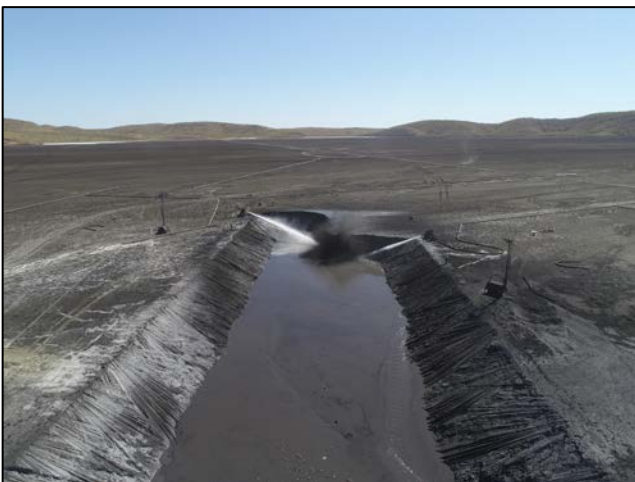
Figures 4 & 5: Hydraulic miners cutting in the initial channel near the inlet to the Slurry Winning Pontoon
