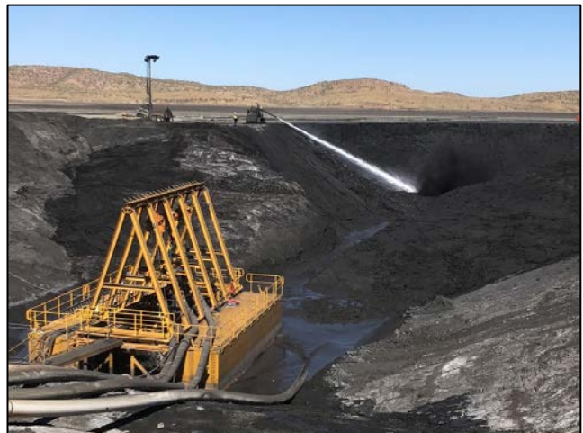
Figures 2 & 3: Aerial view of the Hydraulic Mining Operations Centre and mining progress during August (left) and tailings extraction by the Slurry Winning Pontoon (right)
