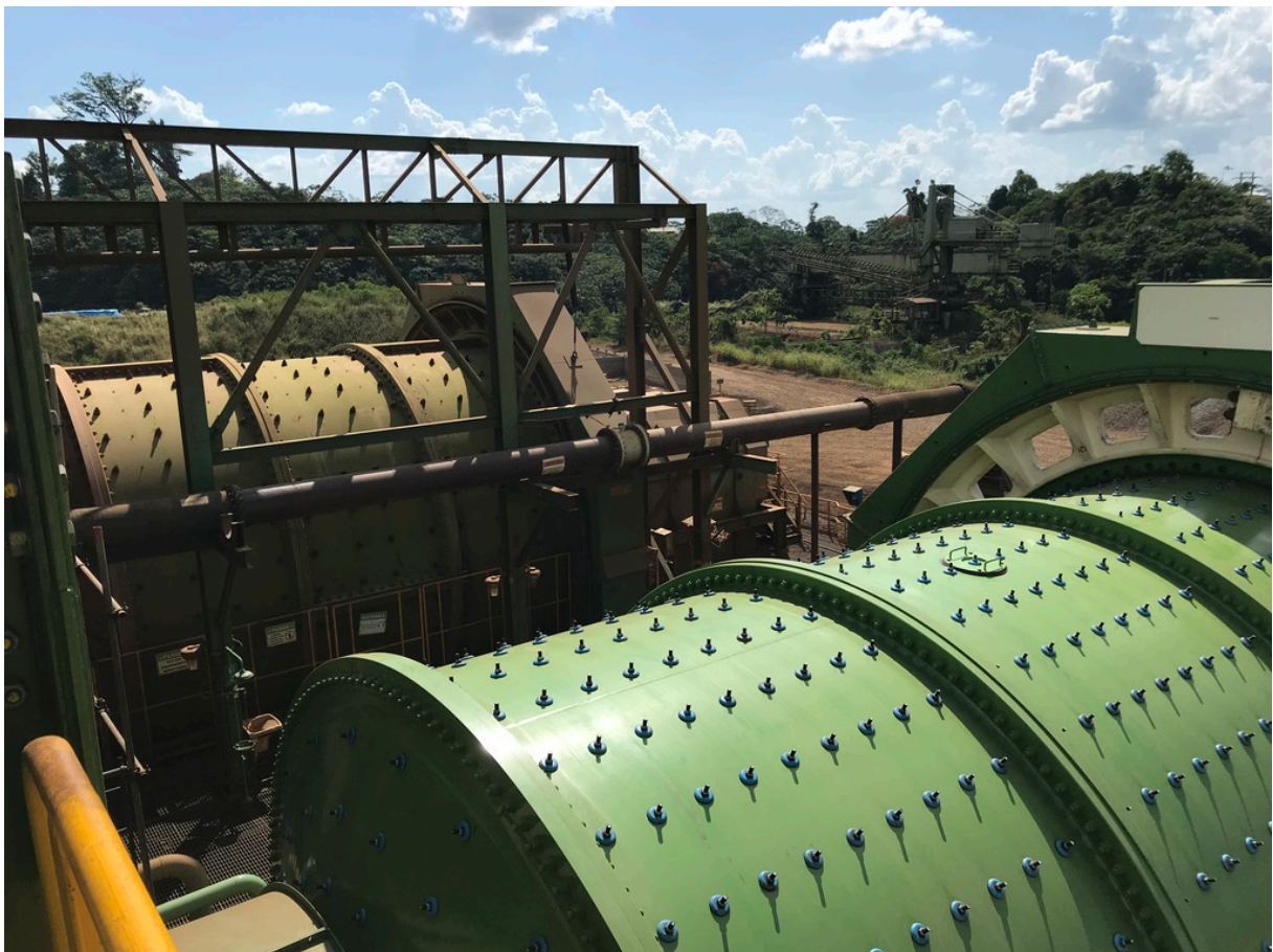
Figure 3. Ball mill in foreground, SAG mill in background
