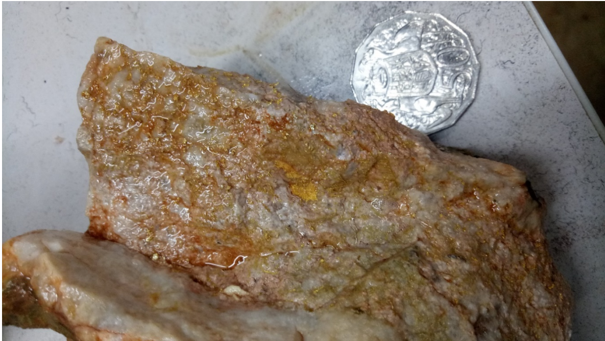
Figure 1 – Quartz vein sample showing gold mineralisation
