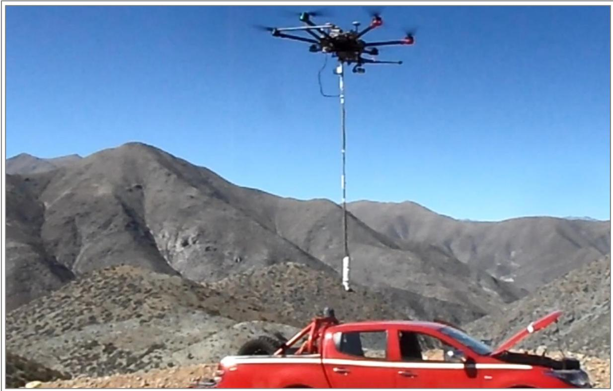
**Figure 3 | Drone and Aeromagnetic Sensor - Joshua Survey (in progress)**
