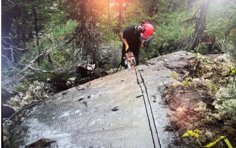
Image 3: Geologist on site at the Lac Rainy Graphite Project preparing the cut for a channel sample on an outcrop of mineralised graphite
