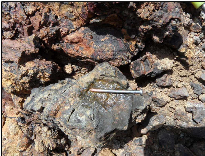
Photo 1: Extensive stockwork present at the Samuel Project containing limonite after sulphides 1 .
