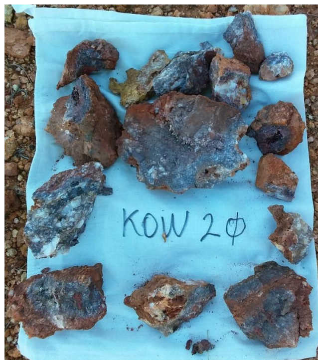
King of the West. Gossanous and fault brecciated vein quartz sample 322499mE 6858909mN
