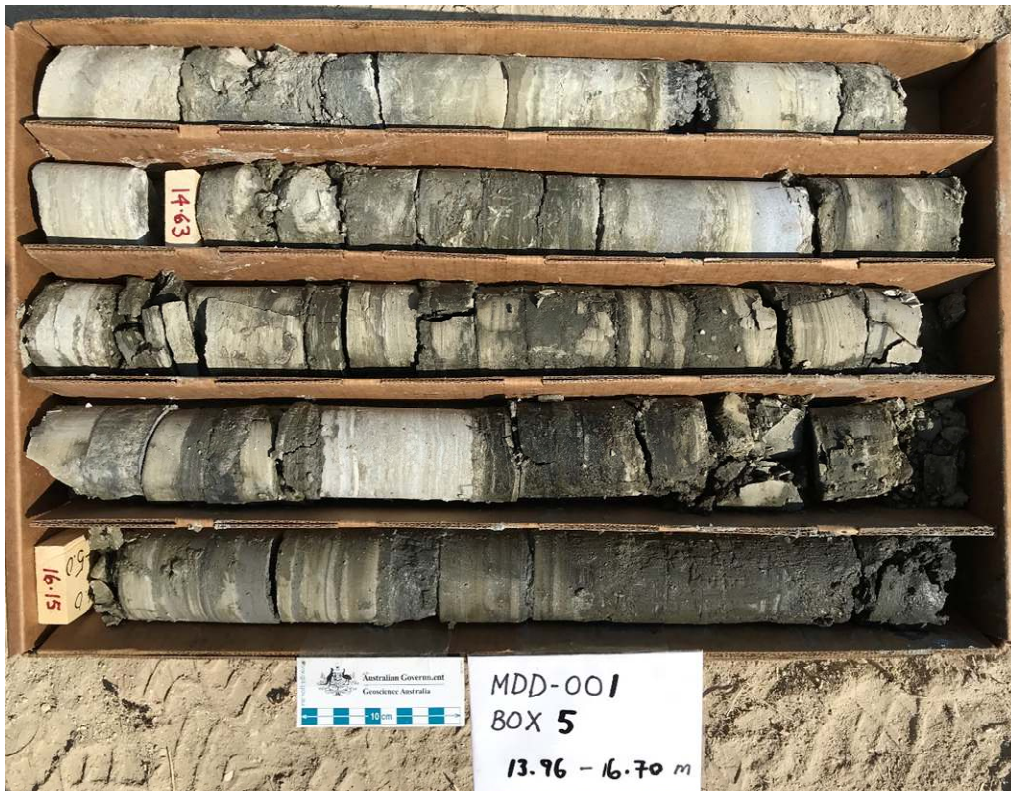
Figure 3 – Example of core retrieved from MDD-01 at McDermitt, showing excellent recovery.
