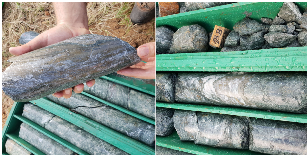
Figure 5: Photos from drill core ALDD008. Left: Quartz (60-70%)-pyrite (30-40%) vein from around 47.7m. Right: Another pyrite-quartz carbonate vein in tectonised gabbro. The vein is located 17.8m down the hole. The sulphide content of the quartz interval in the central core is about 20-30%.
