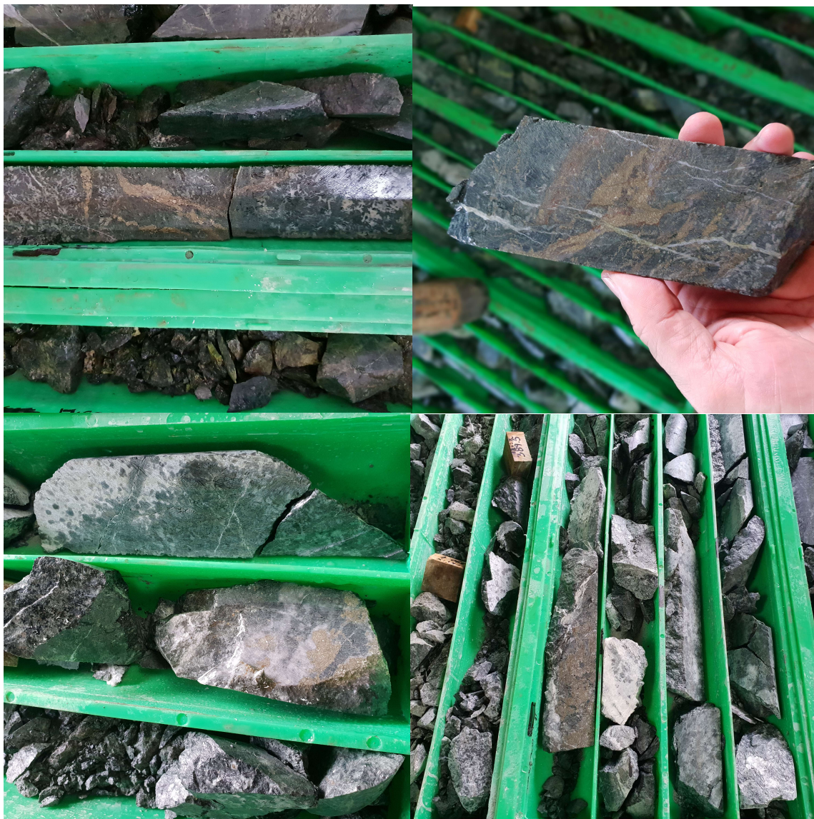
Figure 4: Selected core photos from ALDD003. Top Left: Interval with 10% Pyrite - magnetite veins in gabbro. Top Right: Interval with 5-10% pyrite veinlets in gabbro between 305 to 306m. Bottom left: quartz pyrite vein at 394m. Bottom Right: Interval with a zone of massive pyrite (>80%) and quartz-carbonate veining at 390 to 392m.
