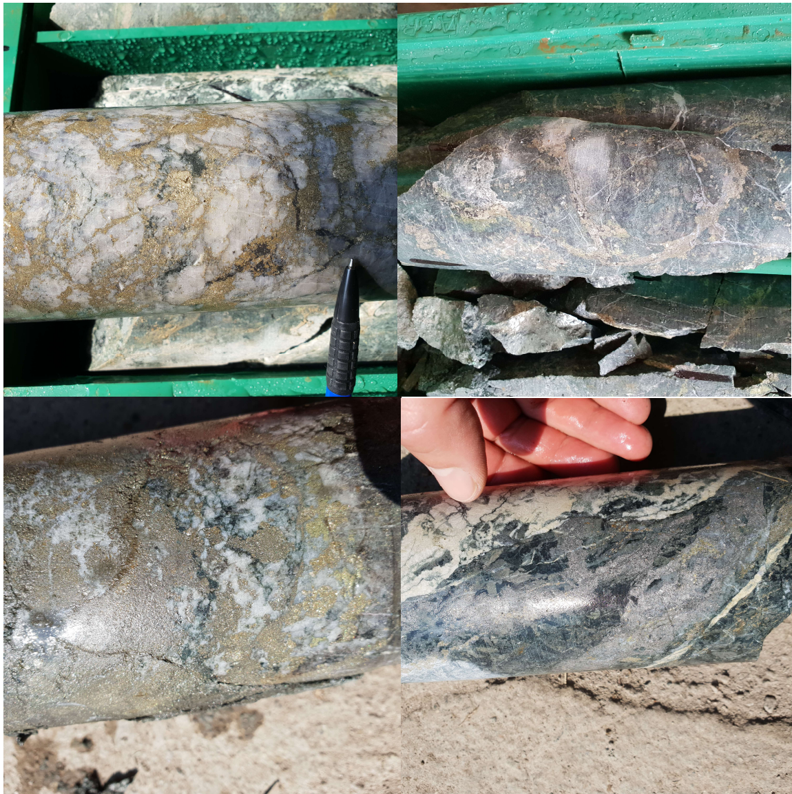
Figure 3: Selected core photos from ALDD004 from 21 to 57m. The photos are selected to illustrate the range of veinlets and mineralisation encountered within the intervals. Top Left: Quartz (60-70%)-pyrite (30-40%)-magnetite (5-10%)-chalcopyrite (<5%) vein interval. Top Right: Pyrite magnetite veinlets, this is the most common style of mineralisation and in this photo the veinlets occupy about 5% of the core interval volume. Bottom left: Semi massive sulphides (70-80% pyrite with minor (<5%) chalcopyrite and 20-30% quartz) Bottom Right: Massive sulphide (80-90%) vein consisting of 60-70% pyrite- 20-30% arsenopyrite and traces (<1%) of chalcopyrite and galena.
