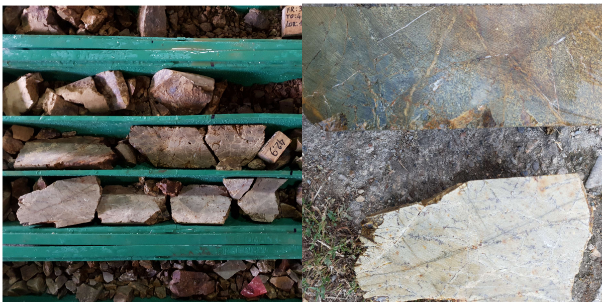
Figure 2: Core from GRDD008 selected from the mineralised interval between 38m to 76m.
