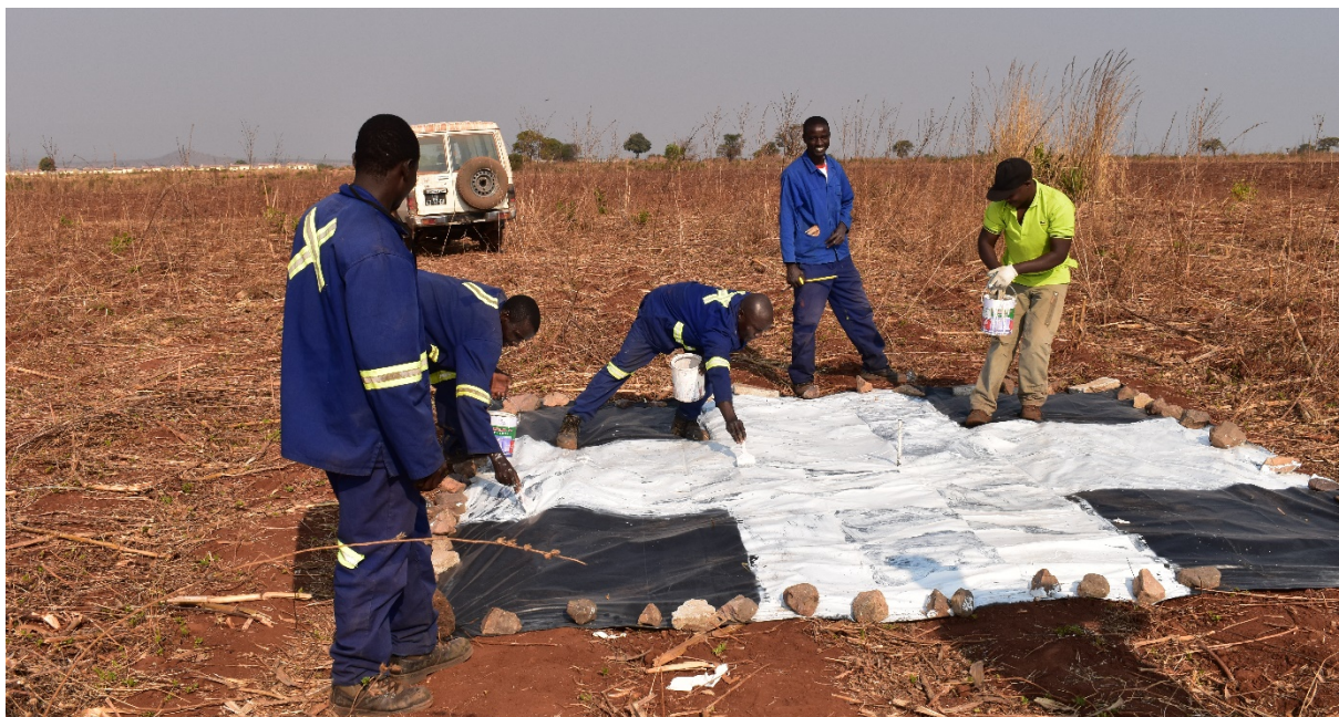
Laying out markers on accurately surveyed Ground Control Points for the satellite digital terrain survey.
