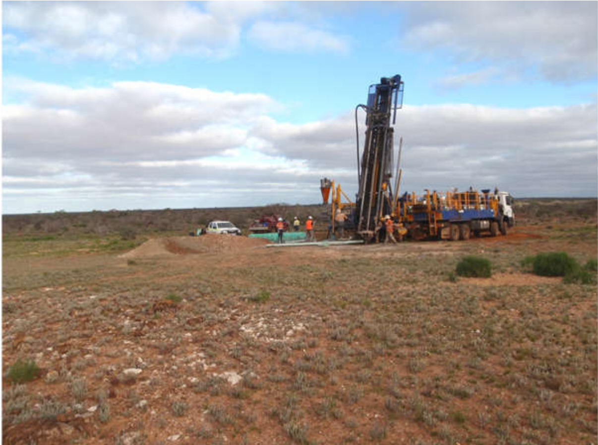
Photograph 2: RMRC 005 and RMRC 006 were drilled at target MG1 from the same drill pad at inclinations of - 50 degrees and -60 degrees respectively. Outcropping mafic schist and white calcrete can be seen in the foreground. A schistose mafic unit over 70m thick was intersected here.
