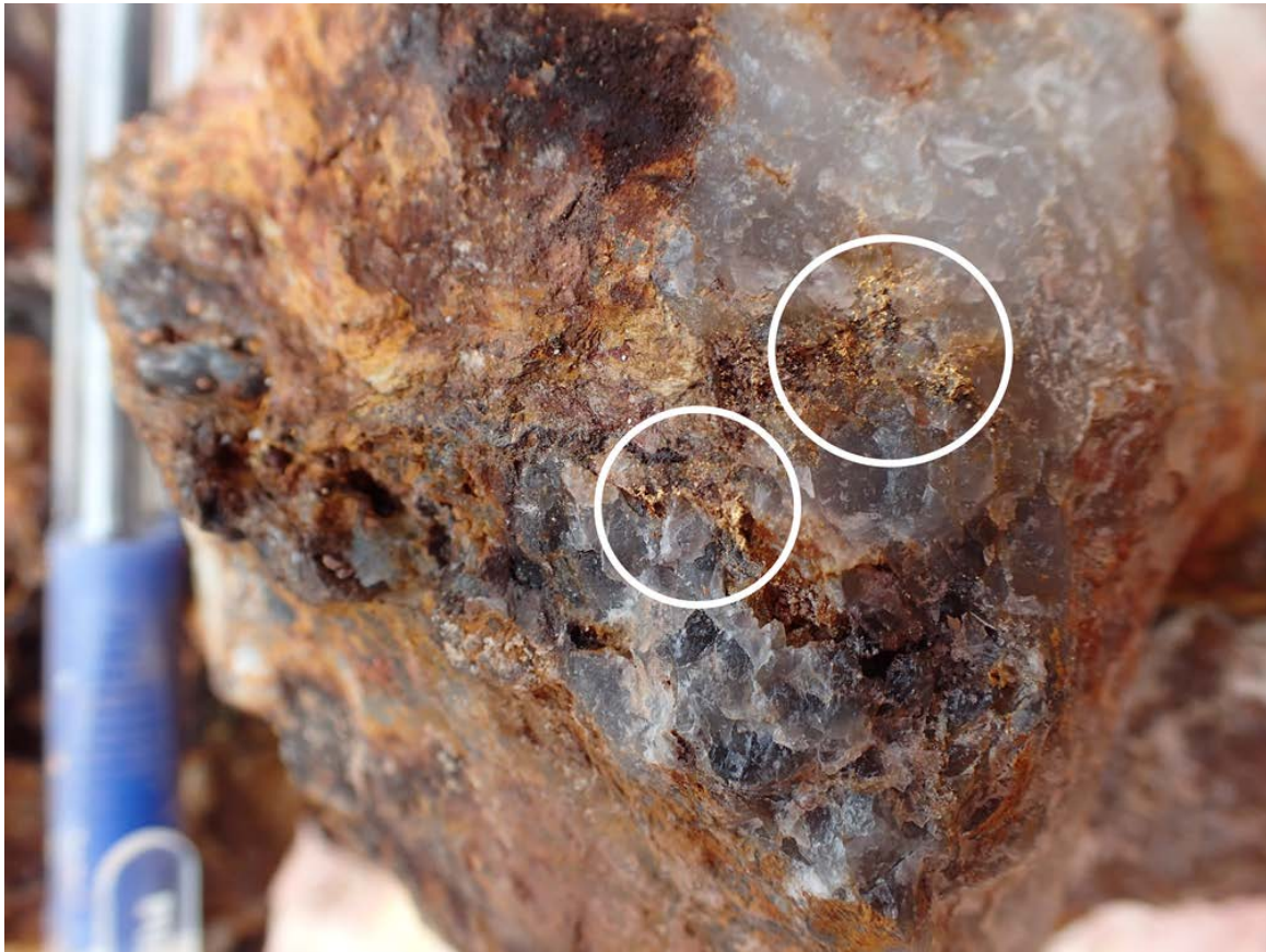
Figure 4: Visible gold in quartz vein from Tallman pit.
