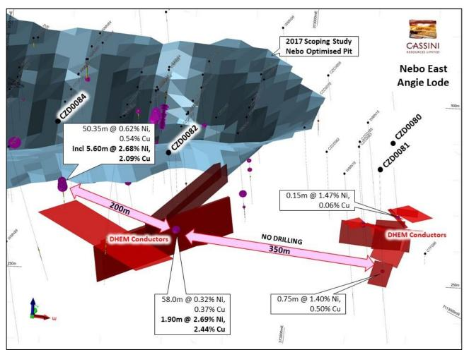
FIGURE 1. Nebo Deposit oblique view showing recent drill results and DHEM Conductors.
