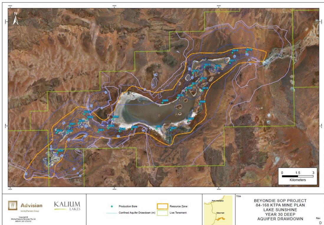
Figure 57: Lake Sunshine Production Bore Layout and Associated Confined Aquifer Drawdown for Scenario 2 at Year 30 [17]
