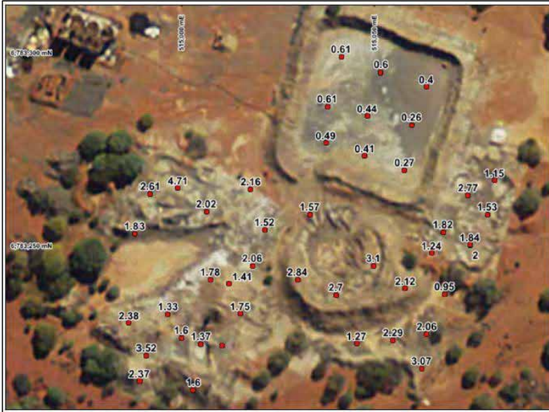
Figure 4-17: Locations of auger holes in the historic tailings area at Reid's Ridge, with gold grades from Apex Minerals
