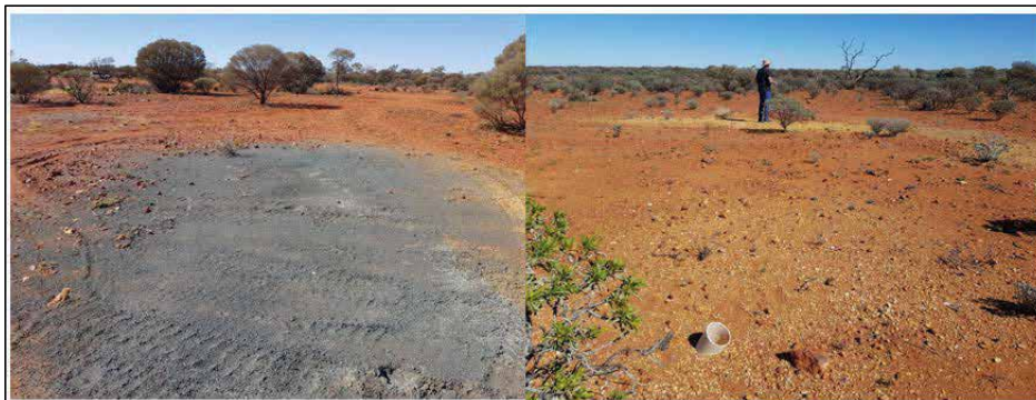
Figure 6-18: Historic drill hole sites, GAR011 drill spoil on left and GAR003 collar pipe
